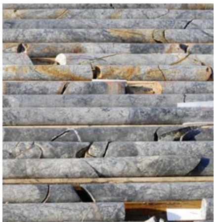
Photo 6. Bottom Coring Samples (USDOI, BOEM, 2013).
