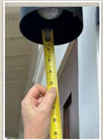
Left to right: sample light fixture, measuring the light baffle width and measuring the light bulb depth. Photos by BHA.
