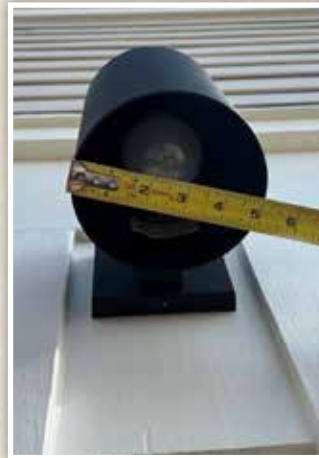
Left to right: sample light fixture, measuring the light baffle width and measuring the light bulb depth. Photos by BHA.
